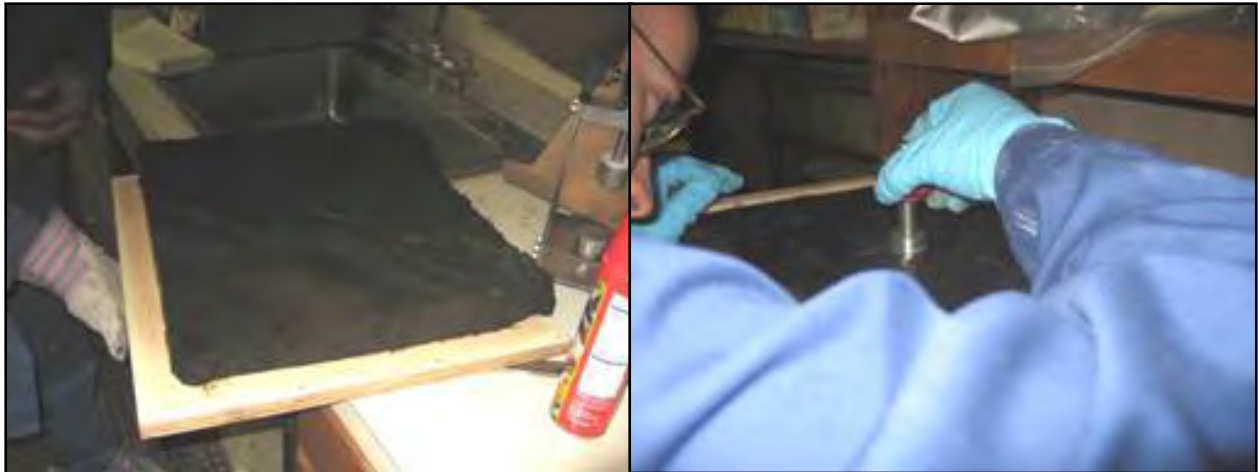
Figure 5.79. Swampy/marsh layer and taking vane shear measurements
