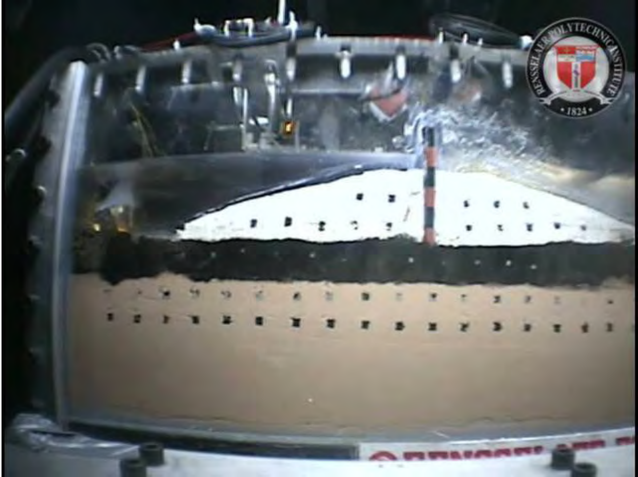
Figure 5.102b. View of RPI Orleans south model at hurricane Katrina flood level
