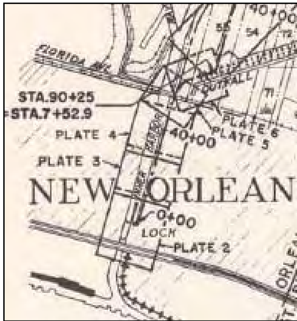
Figure 14-20. Plate 1, DM3Chalmette.pdf Showing Stationing and Soil Boring Locations for IHNC South of Fla Ave
